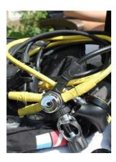
Check your regulator set visually by pulling back on any hose protectors you may have, and ensure that all hoses are intact and haven't started cracking at the points where they bend.
